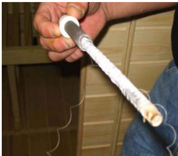
Unapproved heater failure. Fine heater wire can short to non-bonded metal cover plates exposing the user to fire and shock hazards.
